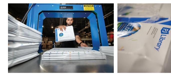
▲ The final step of the book-stuffing process is bundling. Josué Maldonado, a machine operator, uses the blue strap machine to bundle them according to United States Postal Service requirements. In a few days, the USPS will pick up *Kibitzers and Fools* and the rest of the October domestic mailing – 209,307 books in total – for PJ Library subscribers ages 0–8.
